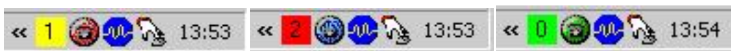
The b+s GraphicServer can be minimized to a tray icon in the taskbar. The colors are a visual alarm to indicate that the number of interactions in queue has exceeded a user defined threshold.
